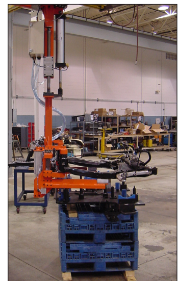
Medium-duty Vertical Balancer handling front sub frame
