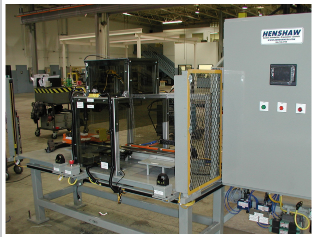
A turnkey control arm inspection system
